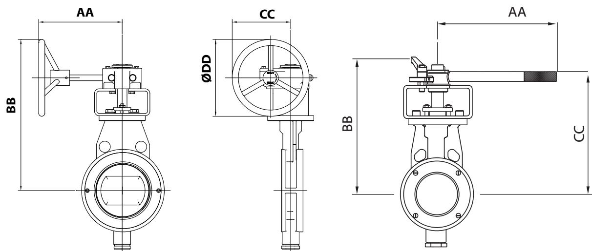
Butterfly valve type VSS with gear unit
