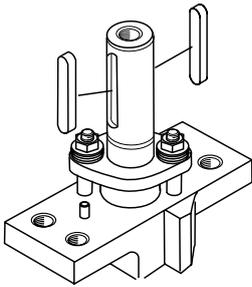
Fig.5-3 Location of the keyway. DN 80-400
