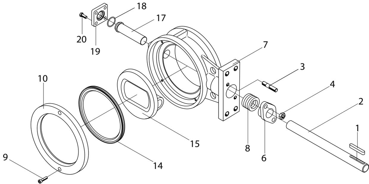
Fig.6-12 DN 200-300, with metal seat
