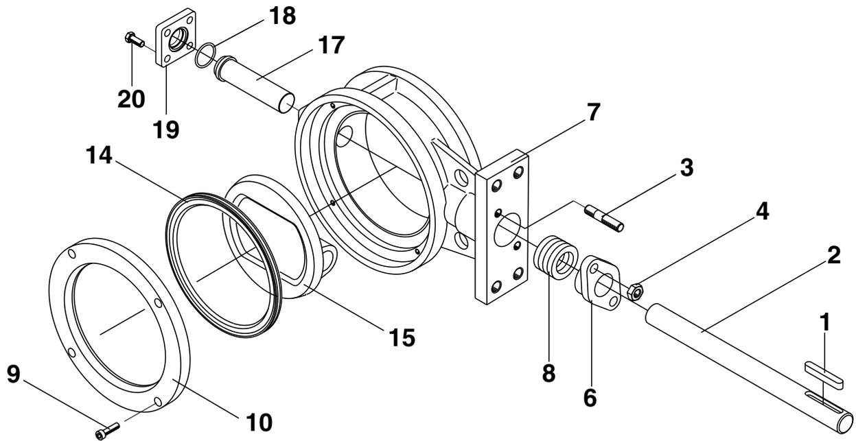
*Fig.6-15 DN 200-300, with PTFE seat*
