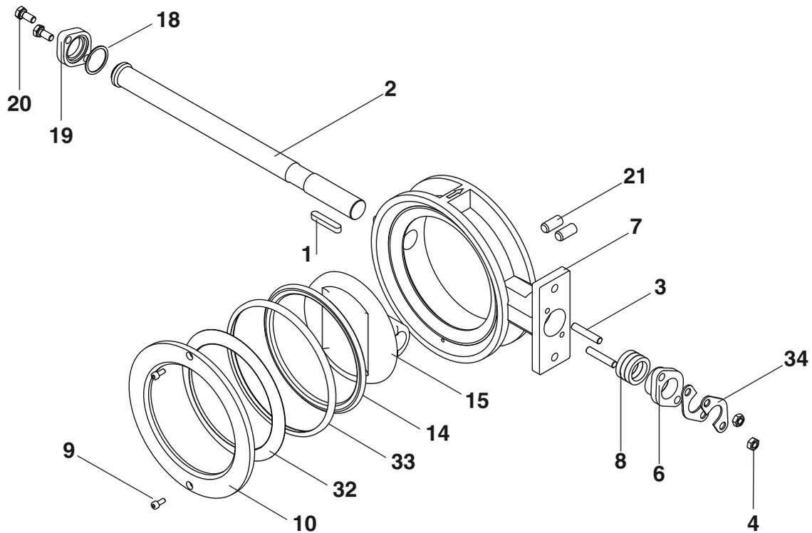
Fig.6-17 DN 100-150, with Fire safe seat
