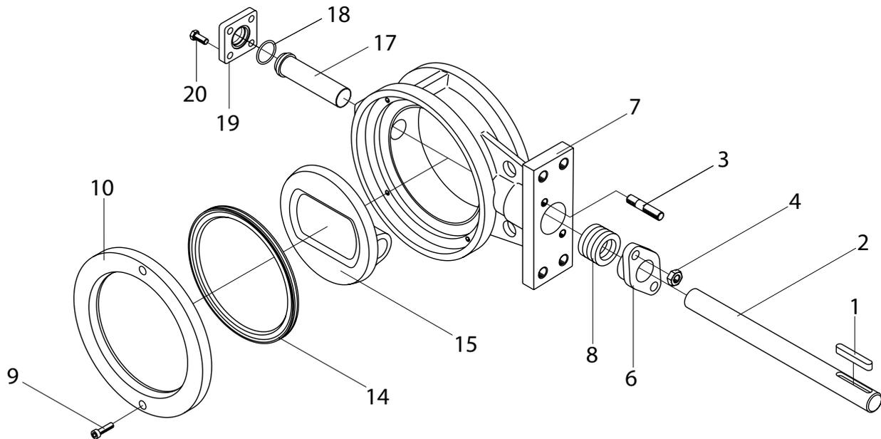
Fig.6-12 DN 200-300, with metal seat
