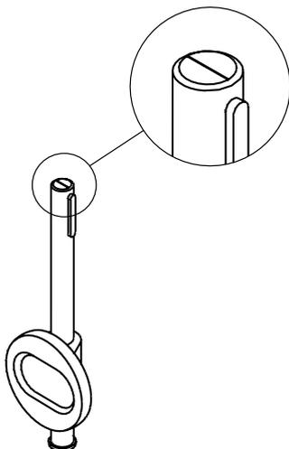
Fig.5-9 Marking (at the end of the shaft)
