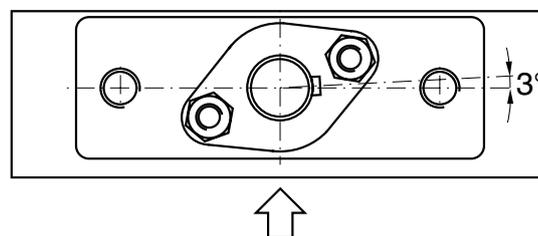
Fig.5-10 Slot angle
