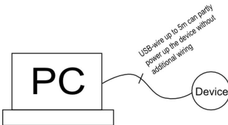
**Figure 7** Parameterization of the device with only USB-connection.
