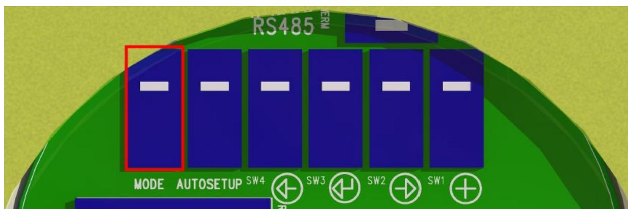
Figure 36: Mode selector key on the main board
