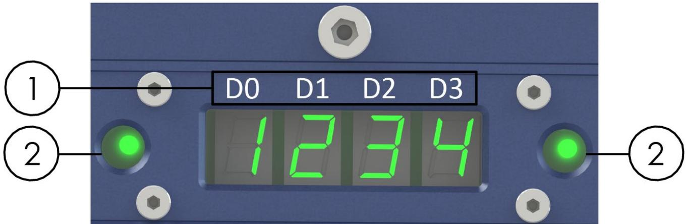
Figure 34: Display on the front panel of the device
