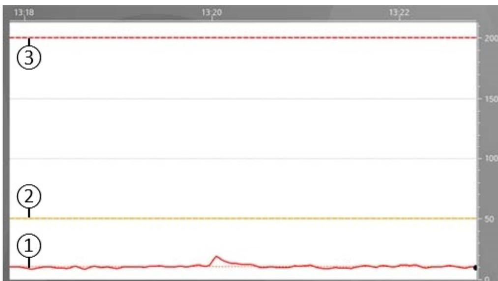
Figure 27: Relation between the output signal baseline and alarm thresholds after Auto Setup
