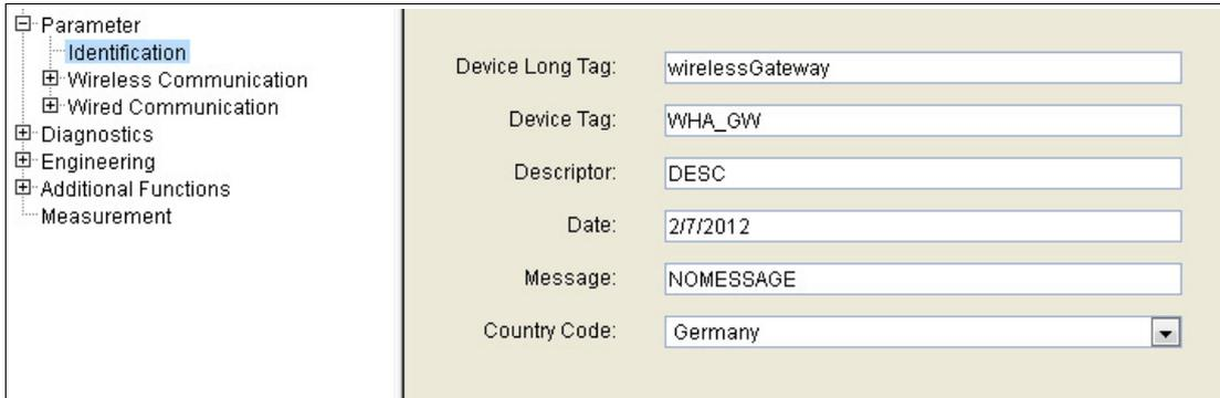
The screenshot shows a web interface for configuring identification parameters. On the left, a tree view shows the navigation structure: Parameter > Identification > Wireless Communication > Wired Communication > Diagnostics > Engineering > Additional Functions > Measurement. The main content area displays the following parameters:
