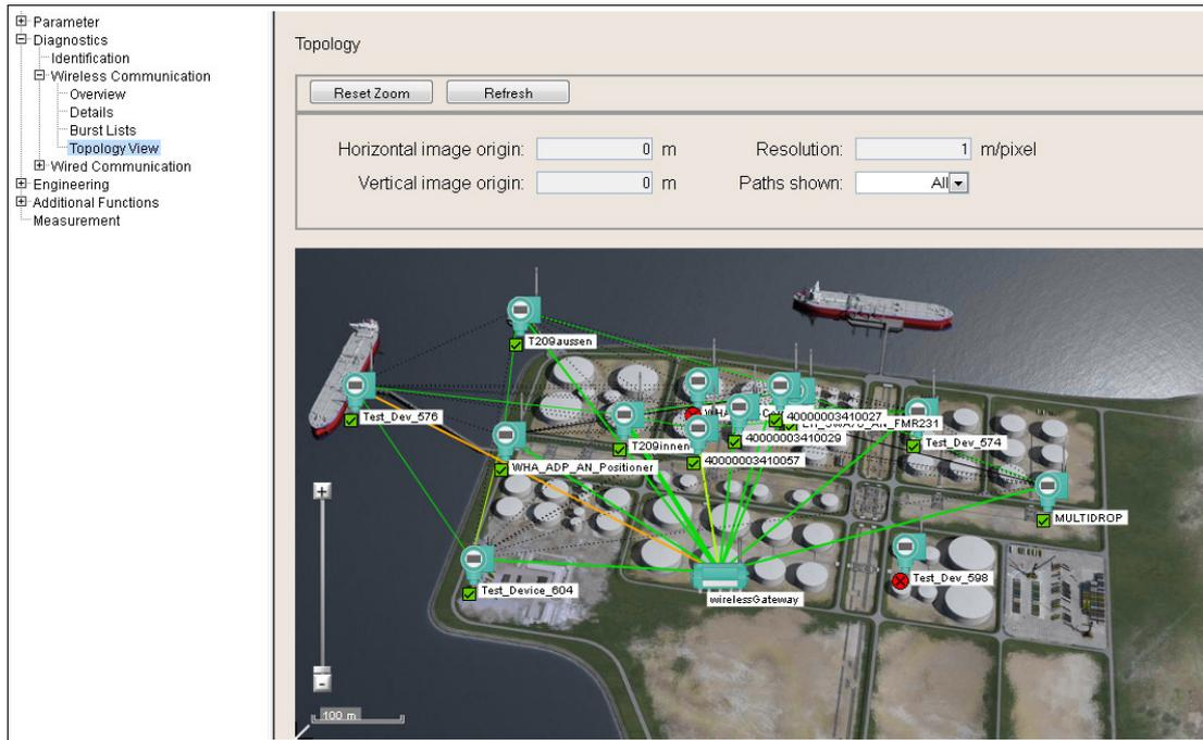
Figure 5.16 Diagnostics > Wireless Communication > Topology View
