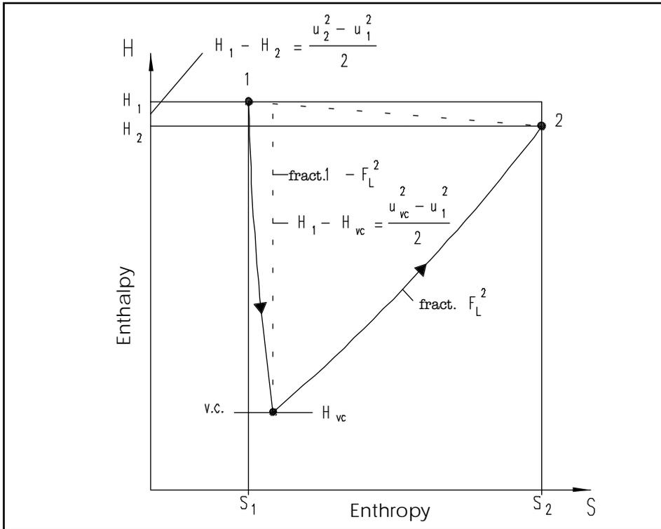
**Fig. 1** Thermodynamic balance inside the valve
