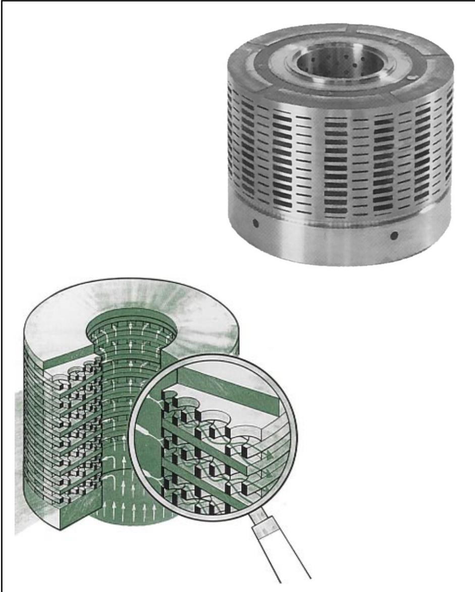
**Fig. 12** *Trim of LIMIPHON control valves of universal multistage/multipath type, provided with labyrinth disk stack. Fluid paths are obtained by overposing disks suitably drilled and mutually oriented.*
