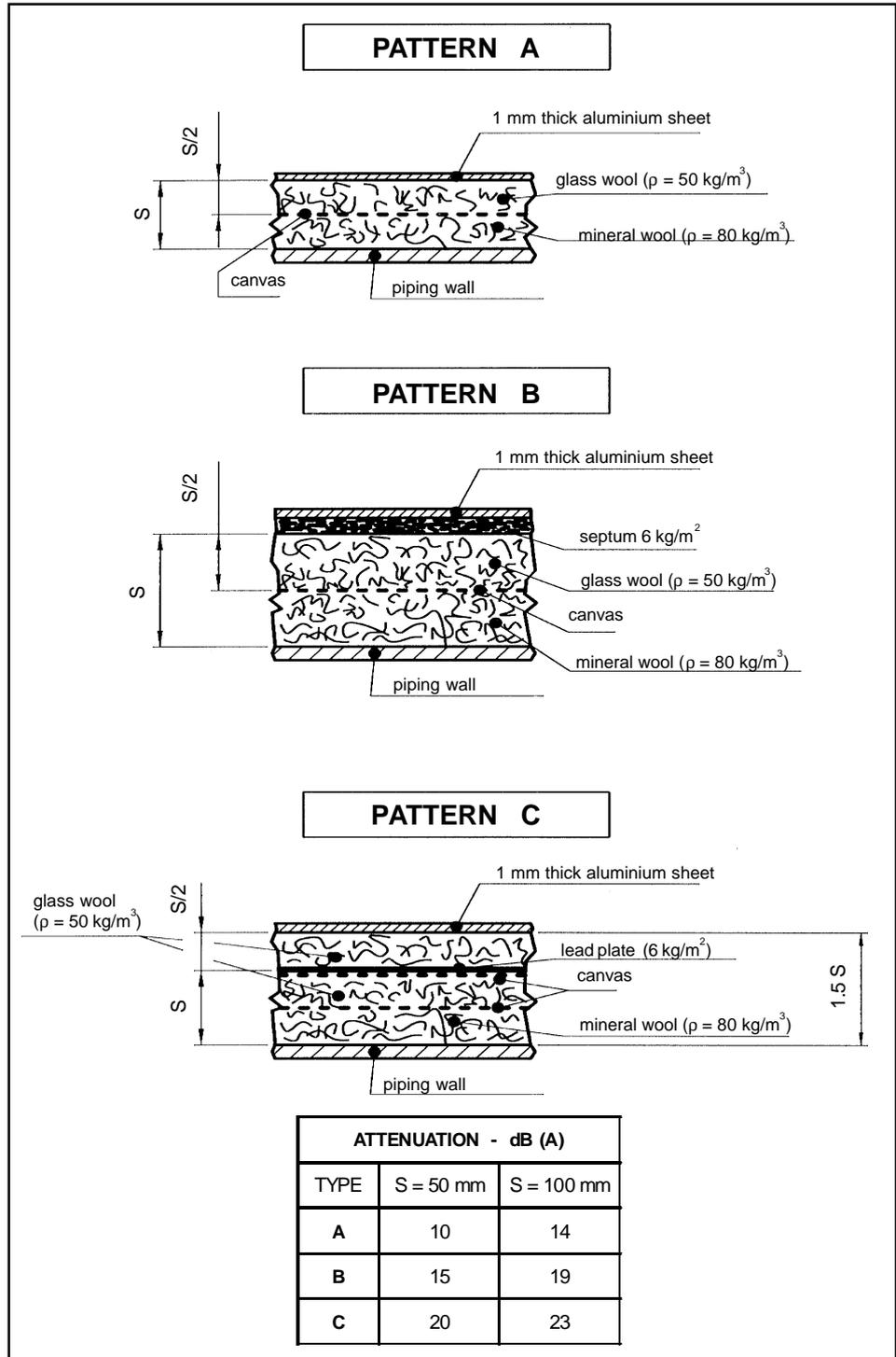
**Fig. 18** Patterns of phono/thermo-insulating laggings of piping
