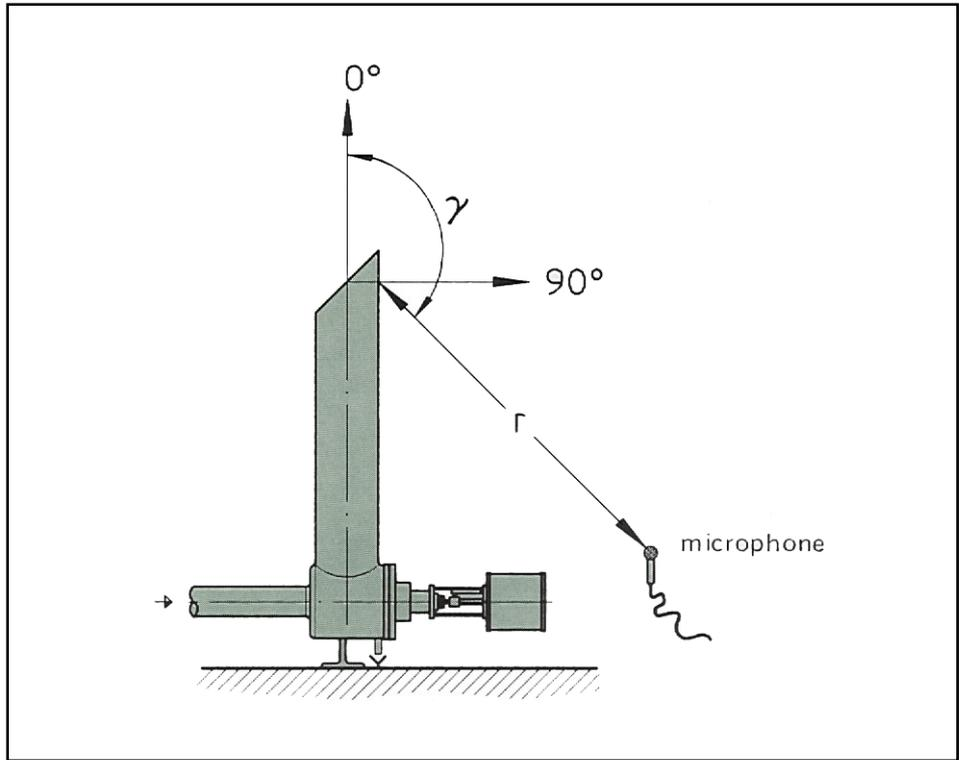
**Fig. 16** *Microphone distance*
