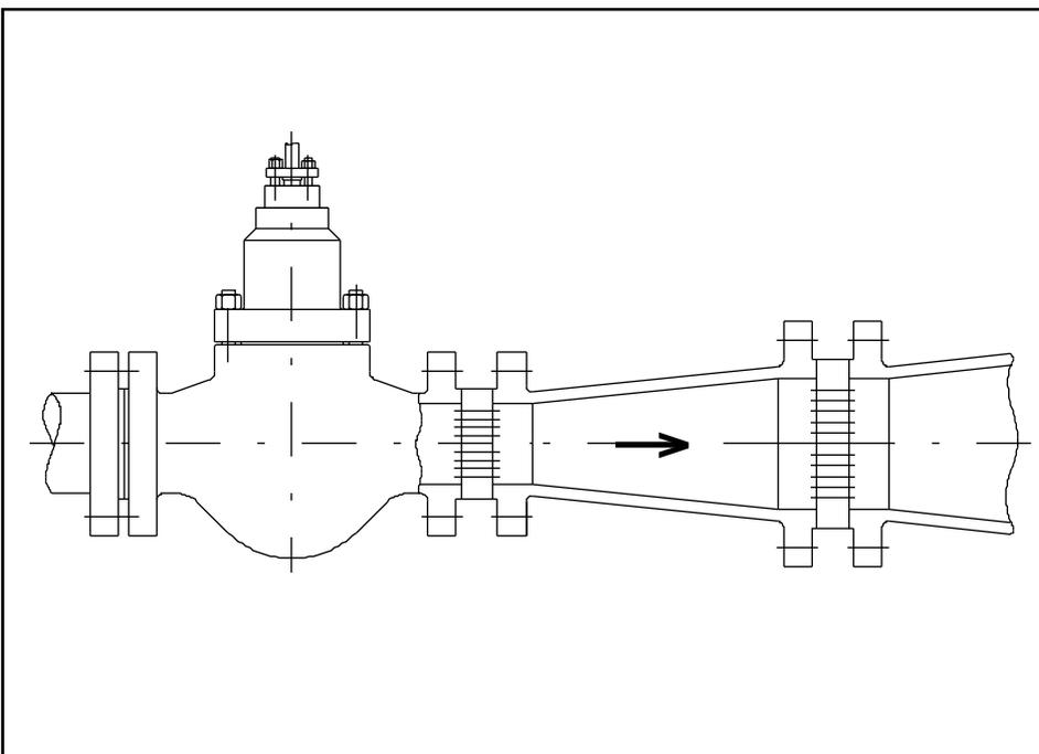
It is possible to try to overcome the first two limitations, mainly the second one, by inserting downstream head losses by fixed sectional area throttles (see Fig. 9).
