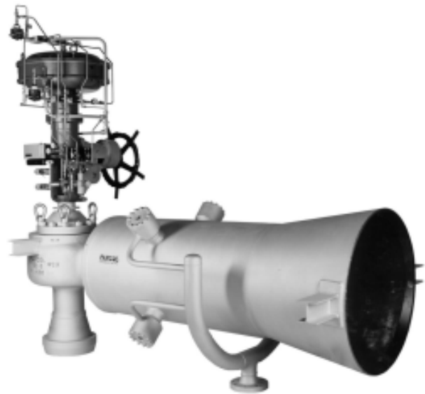
1-9445 Limiphon reducing/desuperheating valve supplied with angle body, bottom inlet and injection chamber provided with multiple LVM type spring nozzles welded downstream.
