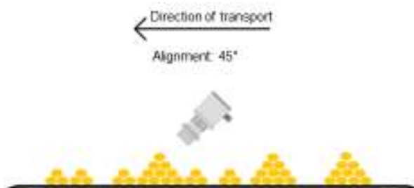
Fig. 2 Installation on conveyor belt
