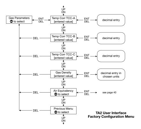
Gas Parameters menu exists for both Gas A and Gas B
