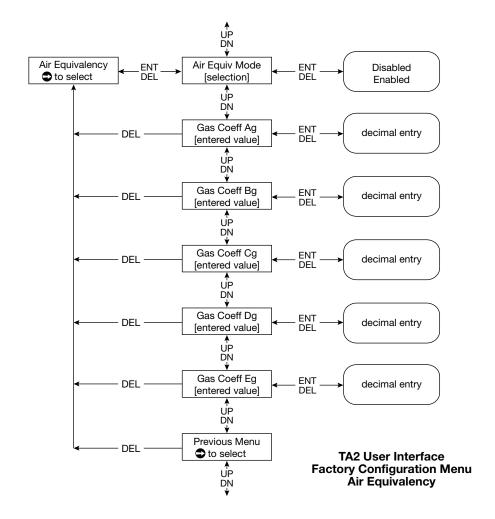
Air Equivalency menu exists for both Gas A and Gas B
