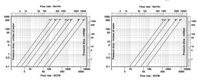
Pressure drop is based on air at +20 °C (+70 °F) and 1 atmosphere (density = 1,2 kg/m³ or 0.075 lb/ft³). For other gases, pressure or temperatures, estimate pressure drop by multiplying value from chart by actual density in kg/m³ (at operating conditions) divided by 1,2.
