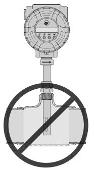
Probe installation into a tee fitting is not recommended
