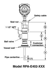
\*Dimension of ball valve if supplied by the factory.
