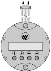
The TA2 has a plug in display (ordered with the unit or separately).
