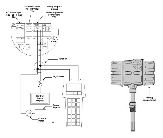
To confirm HART® handheld communications, attach the unit as shown in the illustration. If the communicator reads GENER-IC on the first two lines, then the HART® handheld does not contain the current DDs (Device Descriptions) for the TA2 meter. Contact your local HART® Service Center
