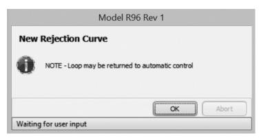
At this point the echo rejection curve can be viewed by selecting Rejection Curve as Curve 2 in the lower left corner of the Echo Curve screen. The Rejection curve will then be displayed as shown in the screenshot below.
