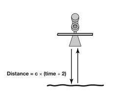
The exact level measurement is extracted from false target reflections and other background noise via the use of sophisticated signal processing. The new PULSAR Model R96 circuitry is extremely energy efficient so no duty cycling is necessary to accomplish effective measurement.
