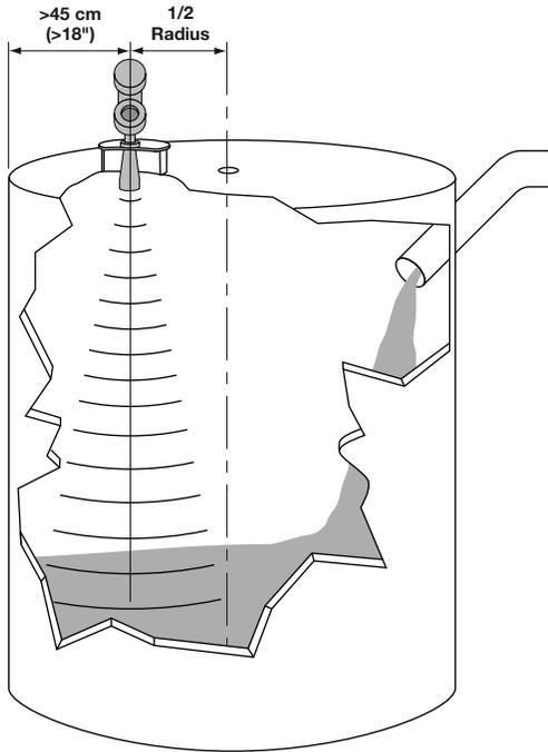
The PULSAR Model R86 Radar transmitter can be mounted to a vessel using a variety of process connections. Generally, either a threaded or flanged connection is used. For information about the sizes and types of connections available, see Section 3.8.2, *Antenna Model Numbers*.
