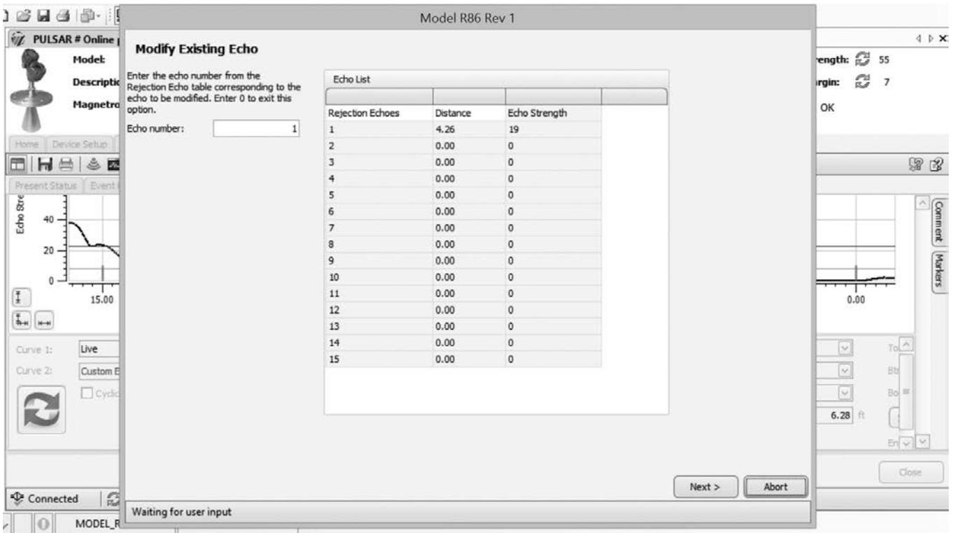
Upon presentation of the Rejection echo list (including the echo amplitudes), along with a display of the present level, select the desired false echo to be modified. (The distance to the echo must be smaller than the distance to the level echo).
