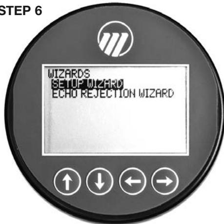
7. After making all of the necessary changes in the WIZARDS menu, press the ↩ BACK button three times to return to the Home Screen.
