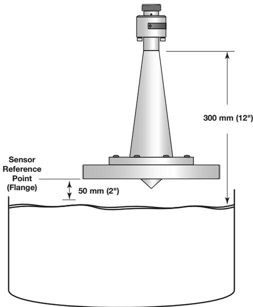
ASME or EN Welded Flange
