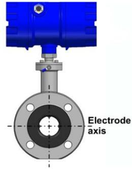
**Figure 12.** Vertical flow going up
