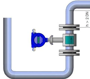
**Figure 16.** Prevent excess vibration
