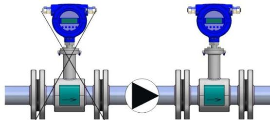
**Figure 10.** Install before control valve
