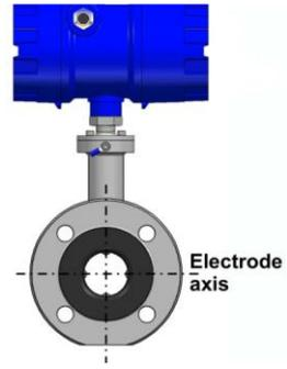
**Figure 12.** Vertical flow going up
