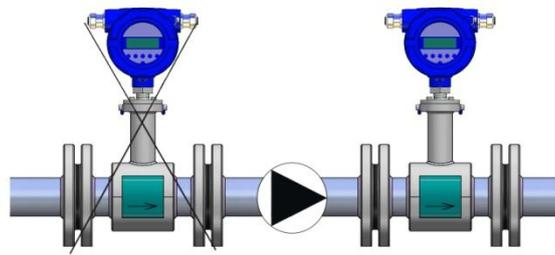
**Figure 10.** Install before control valve
