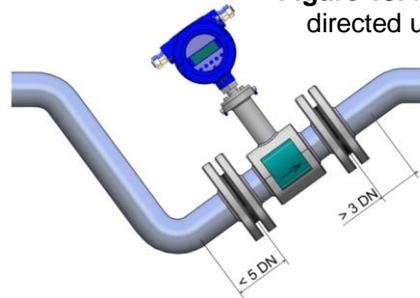
**Figure 14.** No upper pockets or flow going down in vertical section
