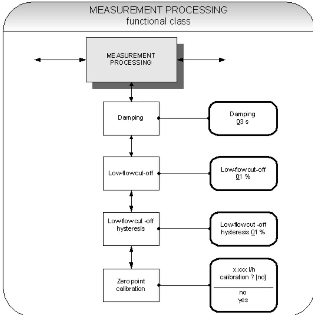
Figure 27. Measurement processing functional class
