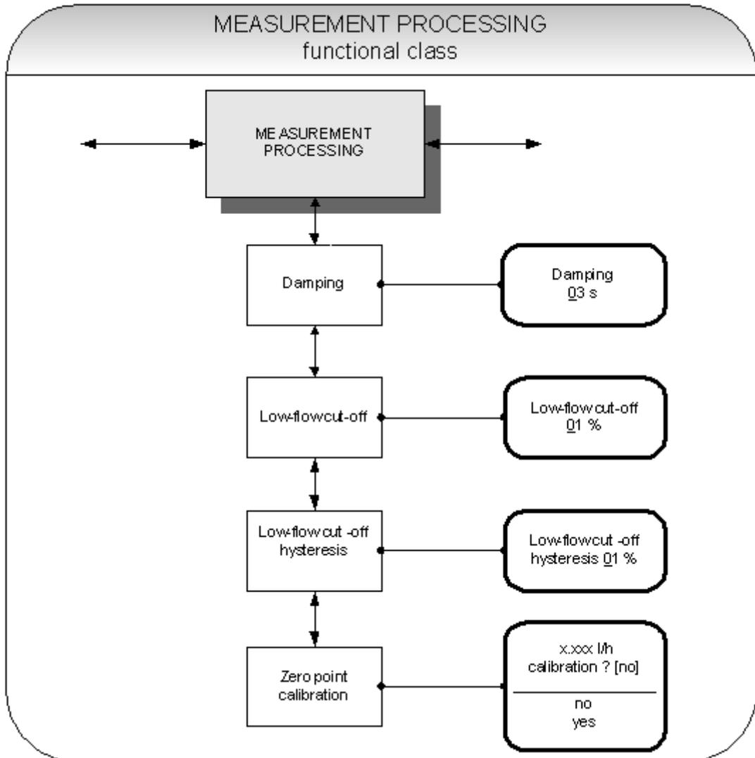
Figure 27. Measurement processing functional class
