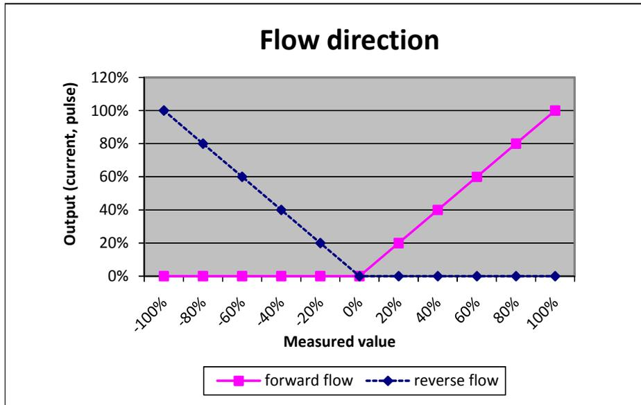
**Figure 36.** Flow direction
