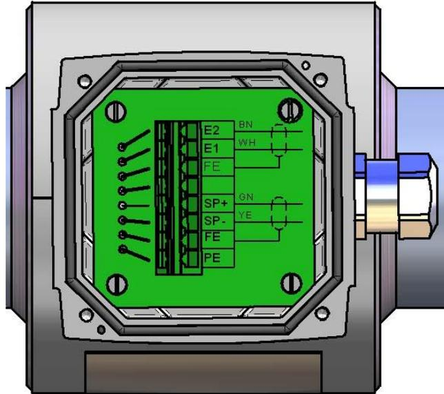
For a sensor with IP68 protection, the inside of the terminal box must be filled with supplied resin GHB1.
