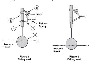
arated by a non-magnetic, pressure tight enclosing tube (5). The switch (2) and magnet (1) are assembled to a mechanism with a swinging arm which operates on precision stainless steel pivots.
