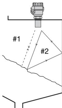
When the distance of the correct echo is entered in P33, the software will move the measuring window and calibrate itself to the proper echo. To determine the distance of the correct echo, either measure the distance with an appropriate device, or use the Echo Map information shown in P70, and enter this value in P33.
