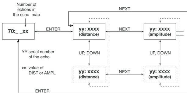
The Measuring Window can be manually moved to one of the echoes displayed in the echo map:
