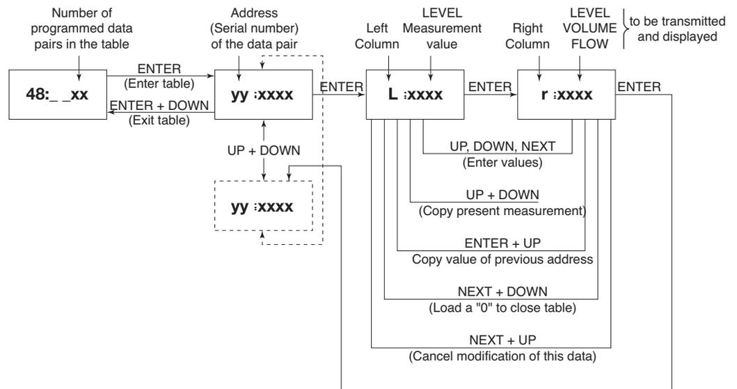
The linearization table must start off with a value being assigned to zero level in the vessel or primary flow element. This zero level is assigned to data pair point 01 as “L: 000.0” and “r: xxxx” filled in with the volume, open channel flow, or level value corresponding to the zero level value.
