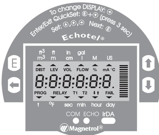
Holding the [E] and [D] buttons down at the same time for 3 seconds allows entry into the *QuickSet* menu. The instructions for entering or exiting *QuickSet* are also printed on a label under the housing cover, just above the LCD module.
