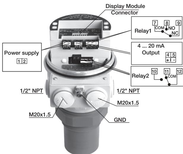
1. Unscrew the housing cover and remove the LCD module to access the removable terminal blocks (TB) position 1–9.
