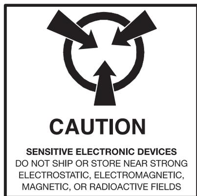
Magnetrol electronic instruments are manufactured to the highest quality standards. These instruments use electronic components that may be damaged by static electricity present in most work environments. The following steps are recommended to reduce the risk of component failure due to electrostatic discharge.
