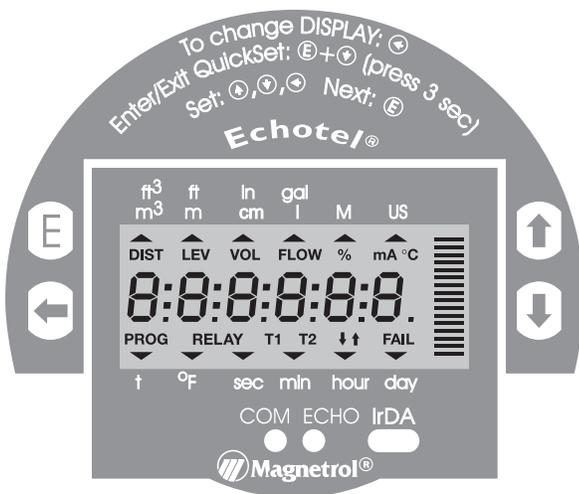
**DIST** = Distance from the face of the transducer to the liquid surface
