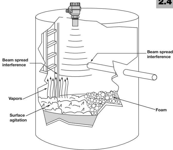
Ultrasonic non-contact transmitters are typically rated for a maximum range in ideal conditions. Experience has shown that maximum range must be reduced for certain factors. Although the maximum range rating is somewhat conservative, each application must be evaluated for specific conditions in the tank.
