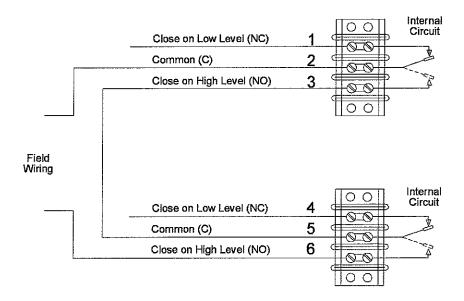
Figure 2. DPDT Wired to be Close on Alarm.
