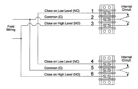
The third method is to wire the two sets of DPDT contacts independently to the Logic Solver. The Logic Solver can then arbitrate between the information on the two sets of contacts. If both sets agree, the measurement is as indicated. If they disagree, then there is a fault in the device. The user can decide the appropriate logic required for the particular application.
