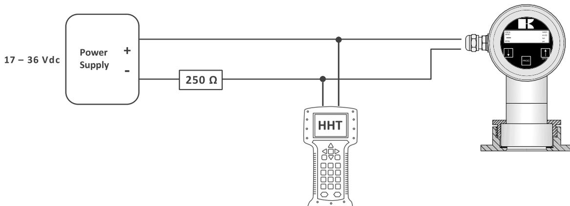
*Option 2: HART® Handheld terminal connected across the loop resistor.*
