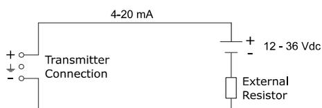
Under the cover ③ you will find the terminal board. The push buttons **Zero**, **Span** and **Prog** are under the other cover ①. External loads must be placed in the negative side of the 2-wire loop.
