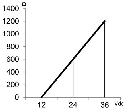
By increasing the power supply, the external load can be increased to 1200 Ω/36 Vdc. (see figure left).
