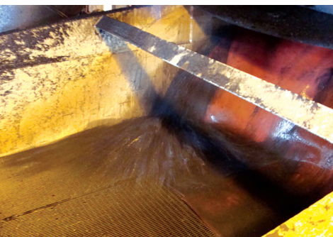
Wet Screens Blocked Chute Detection - Water Sprays
