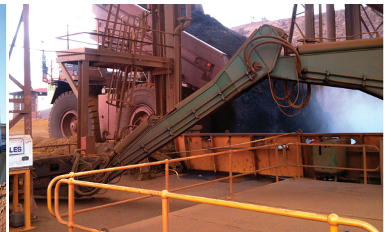
ROM Bins Blocked Chute Detection - Wet / Dry Product / Truck Detection / Water Sprays
