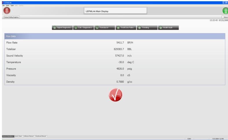
Figure 2-9: LEFMLink 2G Communicating with Transmitter
