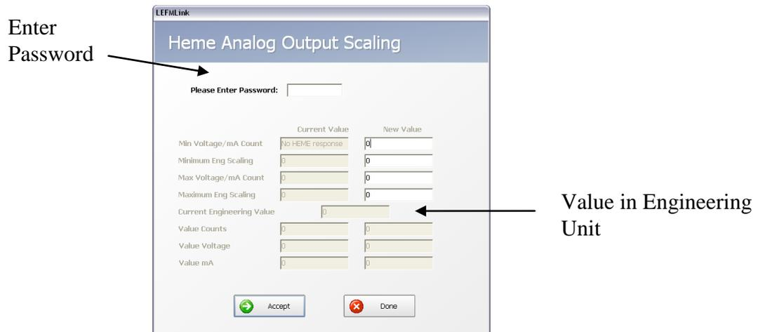
**Figure 6-5: Analog Output Scaling Dialog**
