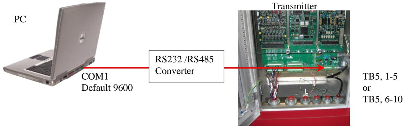
**Figure 2-8: Hardware Connection to NEMA4X Electronics**
