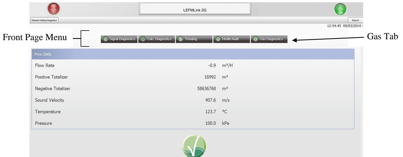
**Figure 8-1 Main LEFMLink 2G screen with Gas Tab enabled**
