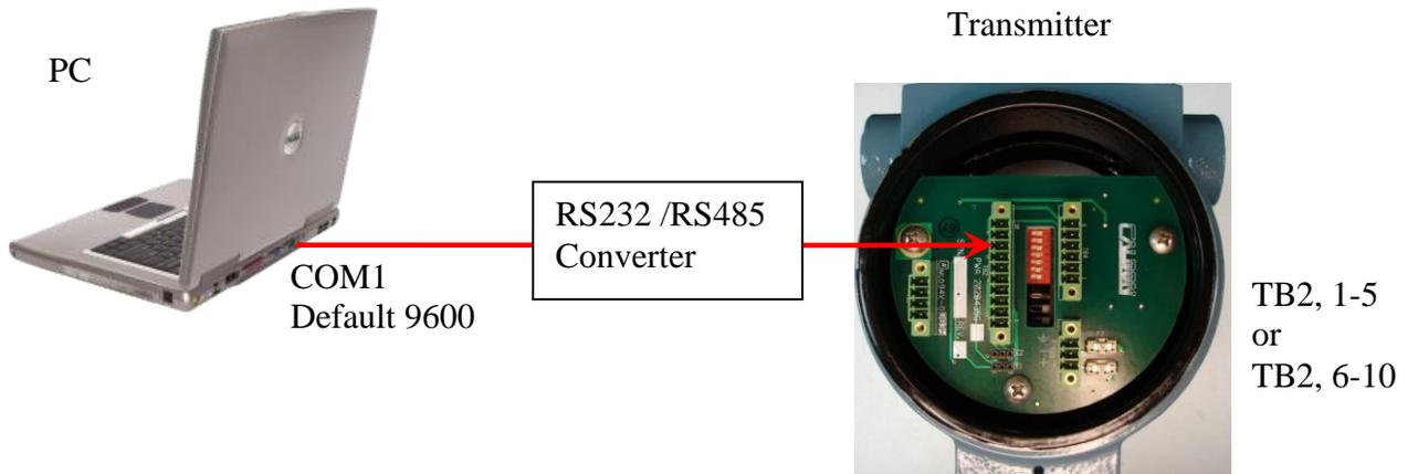
**Figure 2-7 Hardware Connection to Hazardous Area Electronics**
