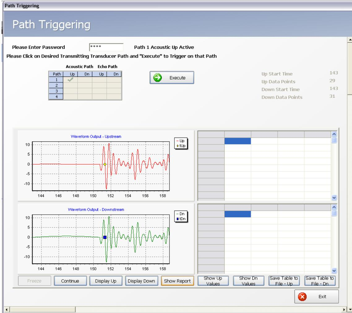
**Figure 6-11: Path Triggering Waveform Displayed**
