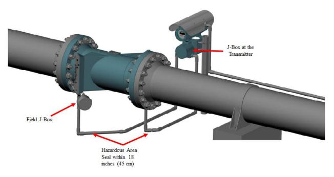
Figure 3.1: Remote Installation of Transmitter from Meter Body
