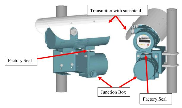
Figure 3.8: Vertical Installation of Transmitter/Junction Box (Sunshield Shown)
