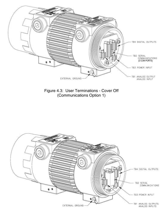
Figure 4.4: User Terminations - Cover Off (Communications Option 2)
