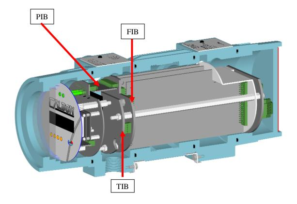
Figure 8.3: Transmitter Passive Components
