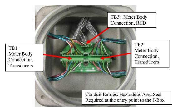
Figure 3.2: 280Ci-R Remote Mount Junction Box Terminations at the Transmitter (Typical)
