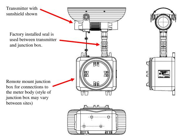
Figure 3.6: 280Ci-R (or 280CiLT-R) Remote Installation of Transmitter/Junction Box
