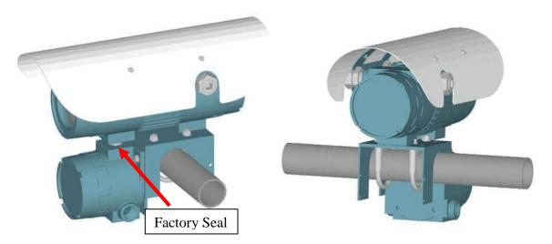
Figure 3.9: Horizontal Installation of Transmitter/Junction Box (Sunshield Shown)
