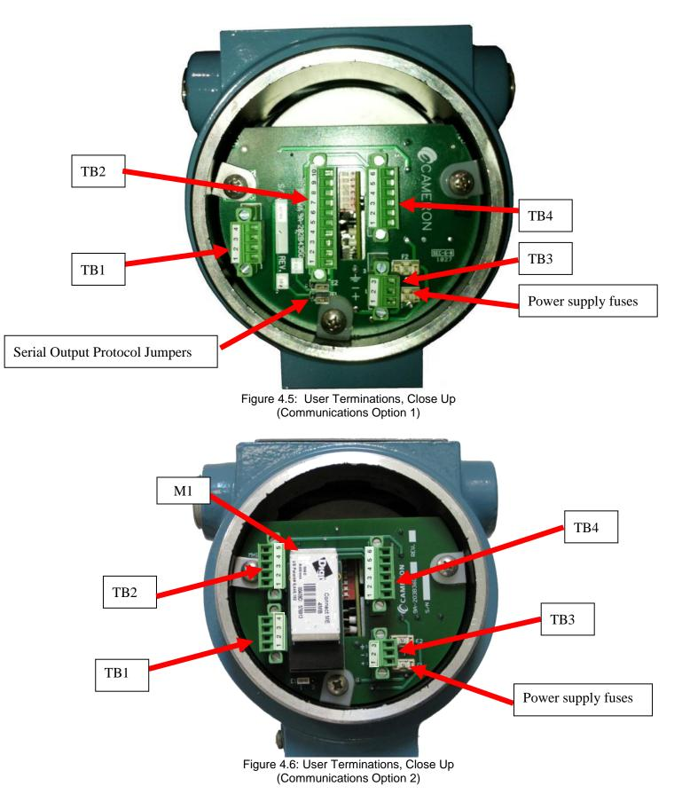
Figures 4.3 thru 4.6 show the location of the transmitter terminations for both communication options. Inside the rear cover of the transmitter there is a diagram of the user connections.
