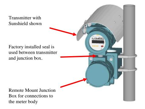
Figure 3.7: 220/240Ci-R Remote Installation of Transmitter/Junction Box
