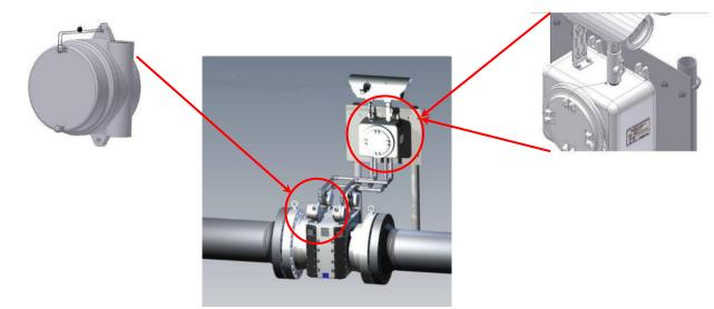
Figure 10-5: Seal Wire for Junction Boxes
