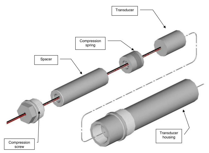
Figure 8.14: Transducer Assembly Construction (half inch housing shown – for the 1 inch housing – the spring and spacer order is reversed).
