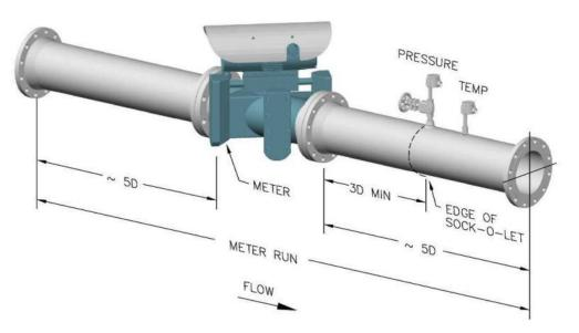
Figure 2.1: 8-Path Meter Best Practice for Installation Hydraulics
