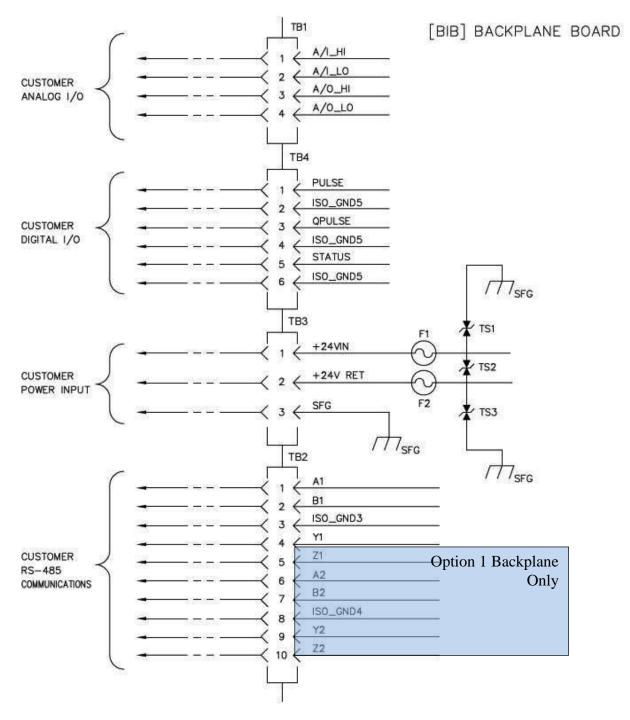
Figure 4.7: User Terminations, Schematic A/I = Analog Input, A/O = Analog Output See Serial Communications Section below for RS-485 definitions
