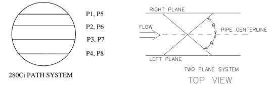
Figure 5.2: Acoustical Path Configurations
