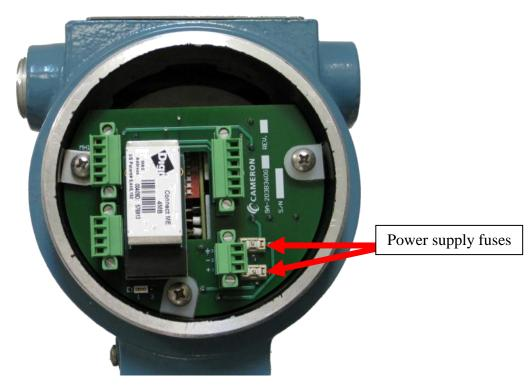
Figure 8.10: Backplane Interface Board (BIB) Fuse Location (Communication Option 2)
