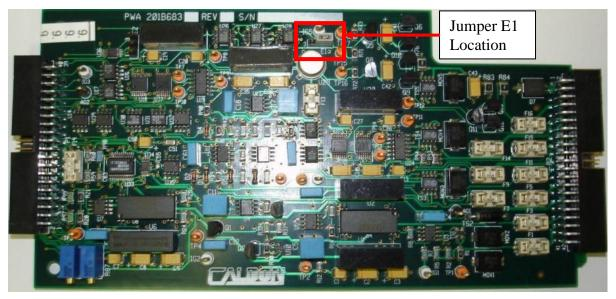
Figure 8.15: Jumper Location to Change Digital Output Voltage
