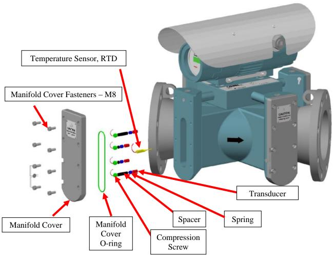
Figure 8.13: Transducer Replacement (note the order of the spring and spacer are shown for 0.5 inch housings)
