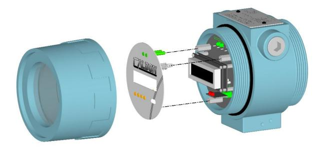
Figure 8.5: Display Cover Removal (Installation)
