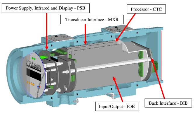
Figure 8.2: Transmitter Active Components
