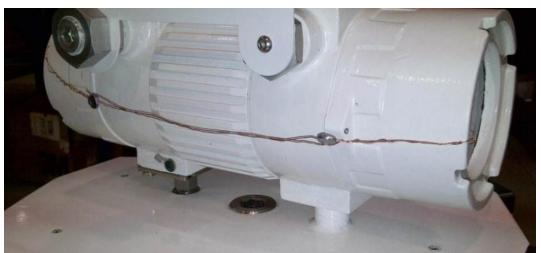
Figure 10-3: Depiction of Seal Wire on Transmitter Enclosure
