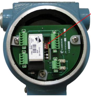
Normal Use: Dipswitches 1 thru 6 inclusive have to be in the "open" position (to the left), dipswitches 7 thru 9 inclusive have to be in the "closed" position (to the right).
