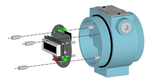
Figure 8.6: Power Supply/Display Removal (Installation)
