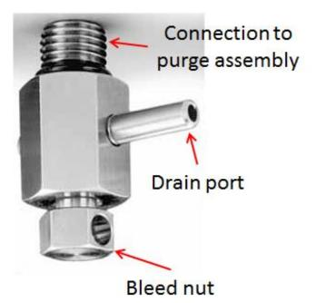
Figure 7.3: Bleed valve on bottom of purge port.
