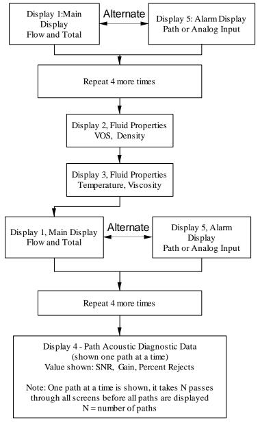
Figure 6.3: Display During an Alarm Condition
