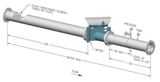
Figure 2-2: 2-Path and 4-Path Meter Best Practice for Installation Hydraulics
