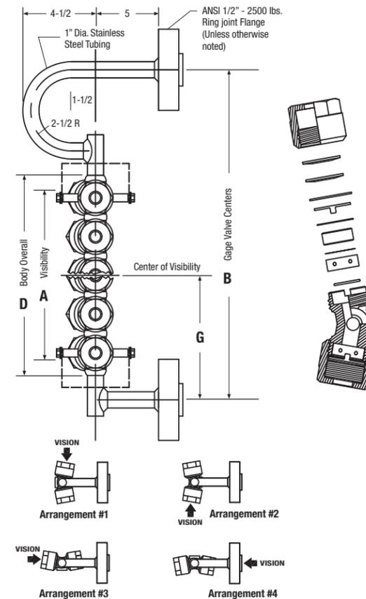
Select an arrangement required. Consult factory for applications with centers less than listed in the chart.
