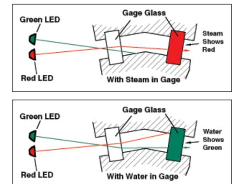
Light does not refract through water on the same line that light reflects through steam. By calculated placement of a light source and gage glass, the Simpliport gage indicates water levels by displaying green ports at water level and red ports for steam above.
