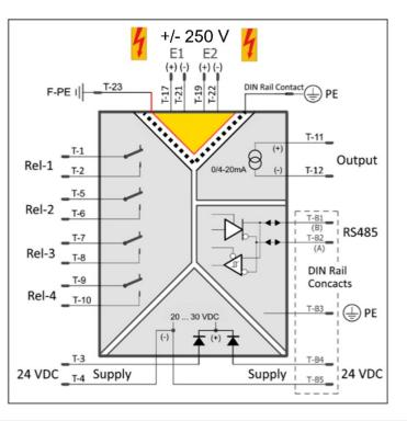
HVT 300-DV Shunt current Measurement HVT 300-DP Balance Voltage Measurement
